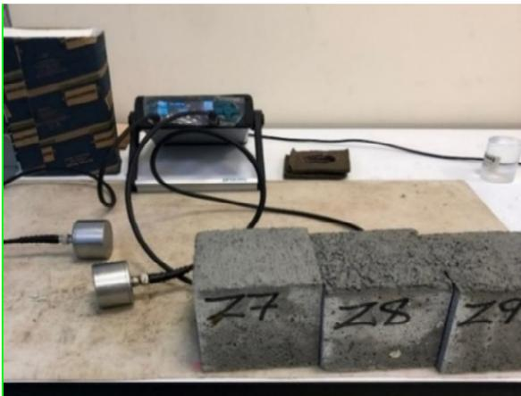
**Figure 2.** UPV test
